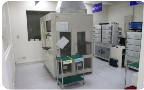
- Thermal cycle SSD testing - 100% burn-in test
